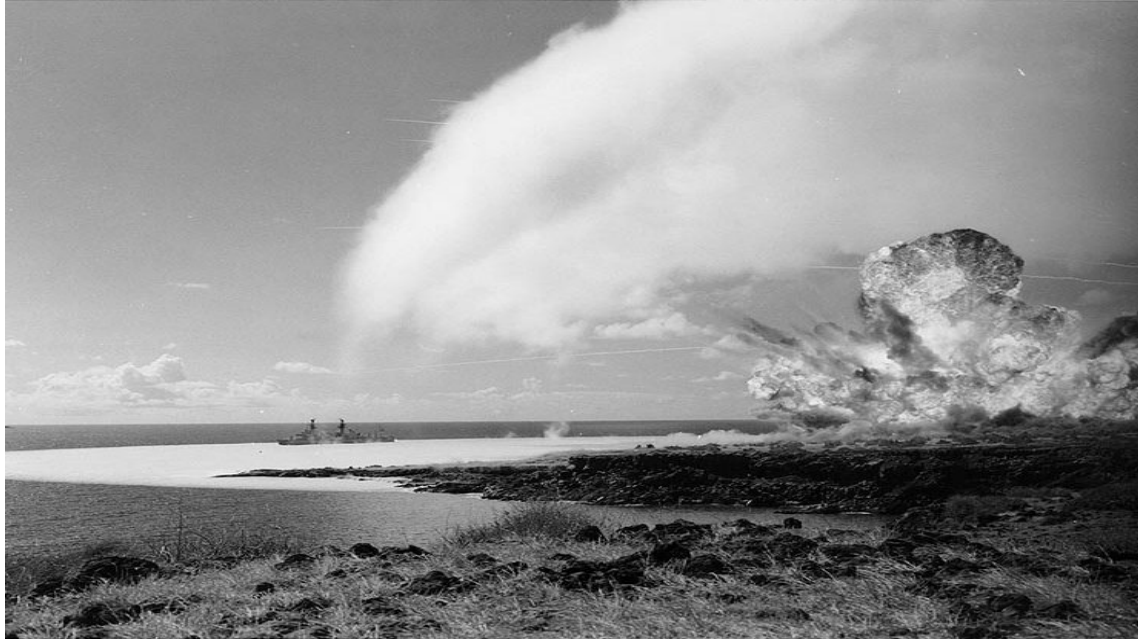
Figure 4.1: The first of a series of three detonations during Operation Sailor Hat in 1965. 500 tons of TNT were detonated to simulate the effects of a nuclear explosion. Public domain image.
